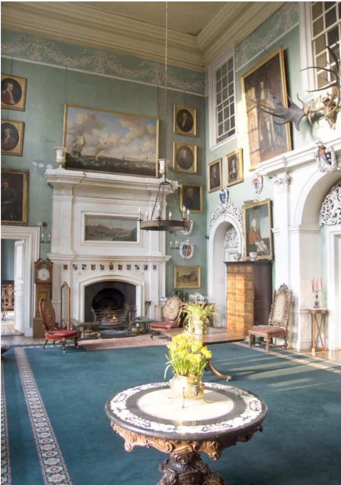
Figure 61: Sunlight streams in through large, single-glazed, west-facing windows, maximising solar gain; however, it also brings about a need to protect historic furnishings and contents from damage caused by both ultraviolet and visible light
