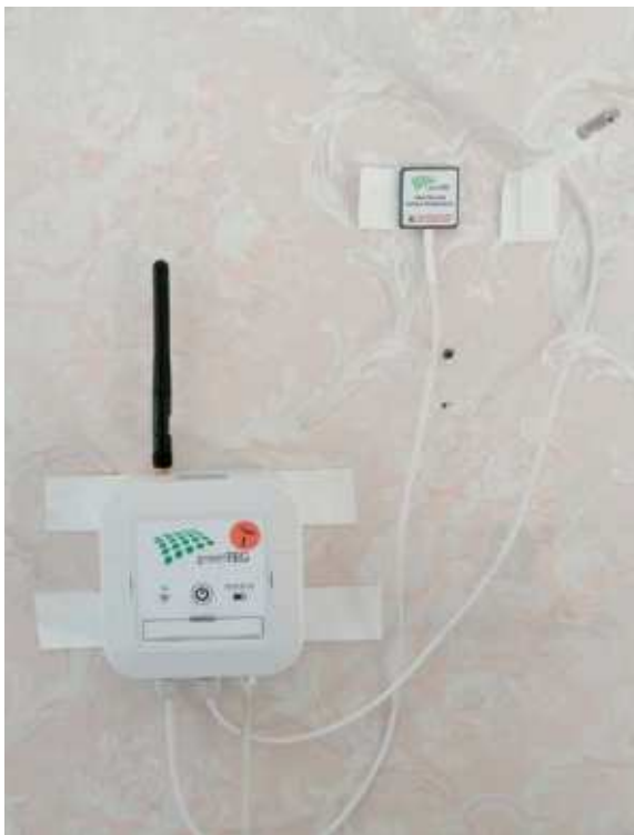
Figure 16: In-situ U-value measurement kit installed on the internal face of a wall (note that the presence of wallpapers may distort the reading)
